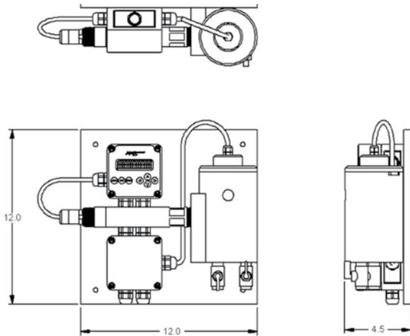
Provides universal conversion of sensor signals and interactive communications for measurement, calibration, configuration and diagnostics. Mounting adapters, junction boxes and recharge kits are available.
